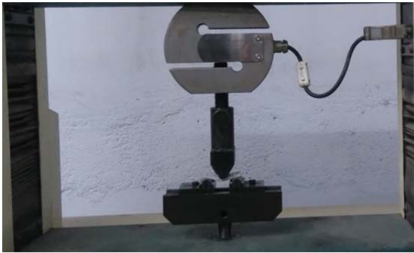
Fig. 3: ASTM D 2344 Short Beam Specimen Configuration.
