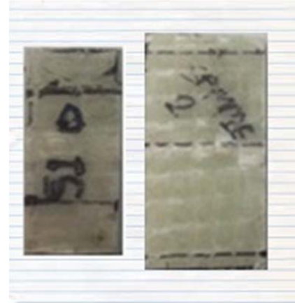
Fig. 8: Samples after test (a) ILSS, (b) Three point bend test
